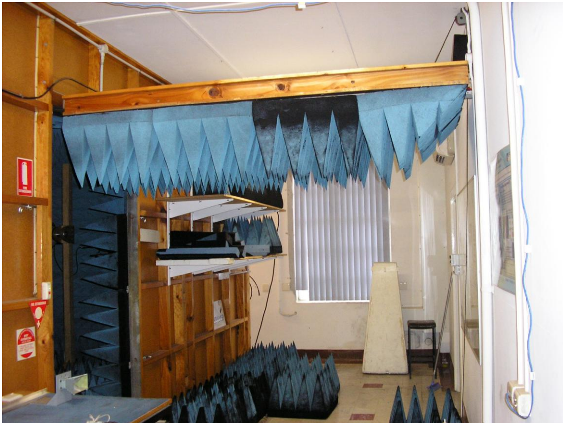
Figure 2. The anechoic chamber door in its fully open position.
